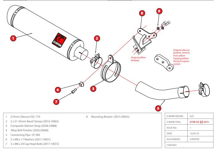
NOTE: ENSURE SCORPION SYSTEM IS CLEAR OF MOVING PARTS AND ALL ORIGINAL FUNCTIONS WORK CORRECTLY.
