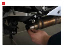
P) Fit Scorpion silencer to the connecting pipe, attach the two springs and using item's 3, 4, 5, and 6 mount the silencer to the pillion foot peg.
