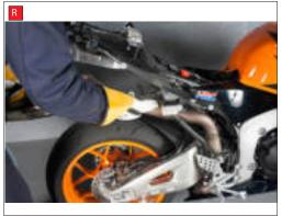
Q) Remove x2 bolts that hold the the O.E silencer.
