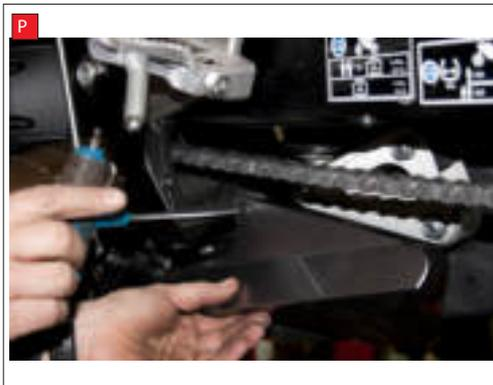
I) Remove O.E silencer mounting bolt, keep this bolt as it will be needed later on in fitting Scorpion Exhaust.
