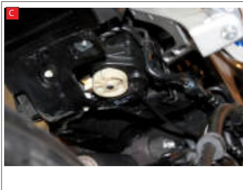
E) Remove the bolt on the belly pan to allow access to the O.E exhaust, save this bolt as it is used later on.
