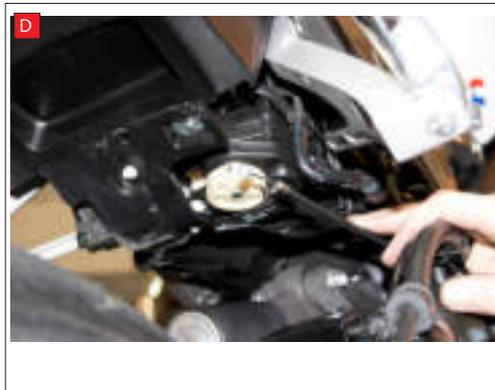
F) Remove the bolt on the other side belly pan to allow access to the O.E exhaust.
