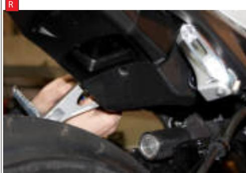
Q) Fit the Scorpion composite fairing, using the line drawing on page 1 to make sure all the fixings are in the correct place, on the top mounting point on the fairing use the O.E bolt.
