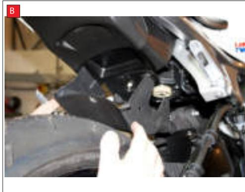
B) Remove back panel to allow access to servo wheel.
