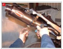
Re-Fit all components (Footrest, Connector Pipe Heatshield, Pillion Footrest, Number Plate & Lights Mounting Brackets, Seat Cowl, Plastic Side Panel and Both Seats) Ensure there is adequate clearance around silencer and link pipe and Scorpion supplied Heatshield is fitted correctly Ensure all original fittings are replaced and all original functions work correctly prior to
