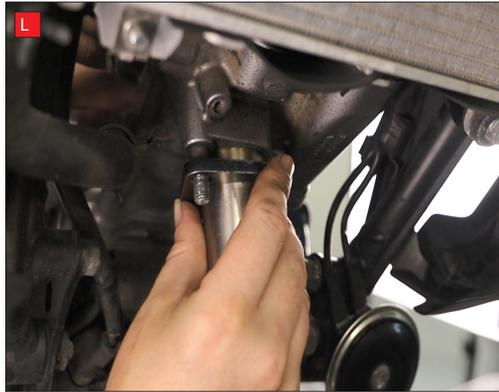
L) Loosely fit the header pipe to the bike.
