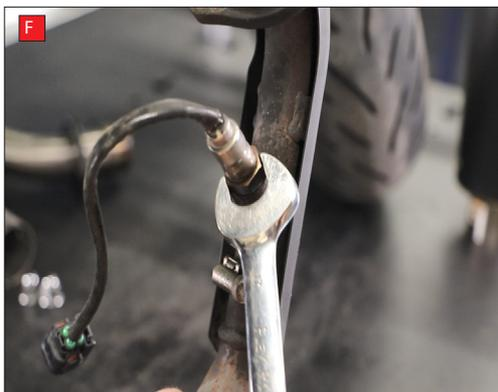
G) Re-fit the lambda sensor in to the Scorpion pipe work.
