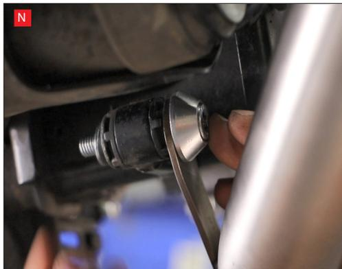
P) Secure the silencer to the connecting pipe using the rubber coated springs.
