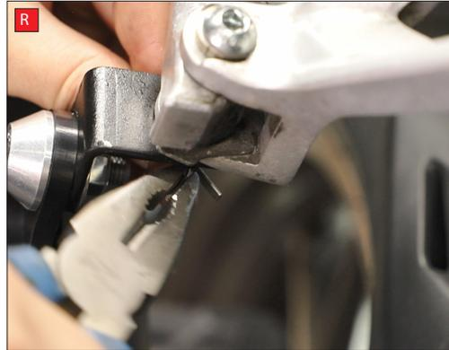
Q) Once happy with the alignment of the exhaust, start from the front of the system working your way back, tighten all fittings.
