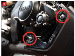
A) Remove the 3 screws on the right side lower front panel and then the 3 on the left side as well.
