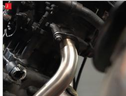
I) If the exhaust gasket has stayed on the engine, remove it now as it's not required with the Scorpion system.
