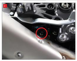
I) Remove the 4 nuts holding the headers to the engine.
