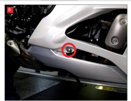
A/B/C) Starting on the right side of the bike, remove the 5 mounting screws for the lower fairing.
