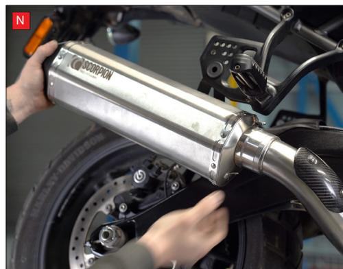
O) Push the original mounting bolt through the rubber on the frame and the new mounting bracket behind it and secure in place with the supplied washer and locking nut. Again, leave this loose for now, you will fully tighten it later.
