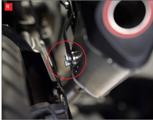
R) Fully tighten the bolts that mount the bracket to the silencer.
