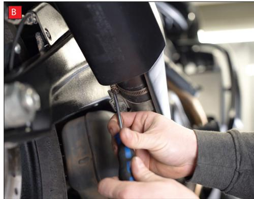
A) Start by removing the screw from the connecting pipe cover.
