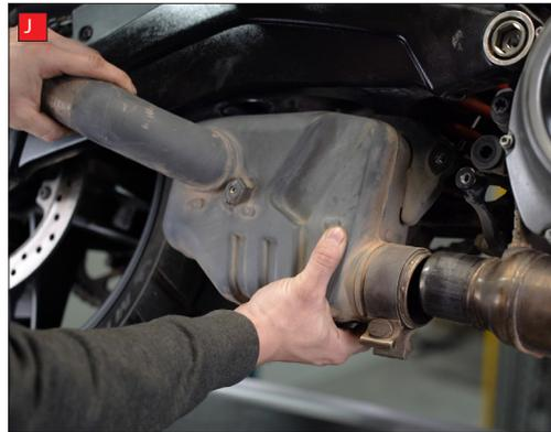
I) Remove the centre silencer mounting bolt.
