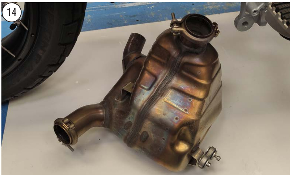
REMOVE THE MIDPIPE
