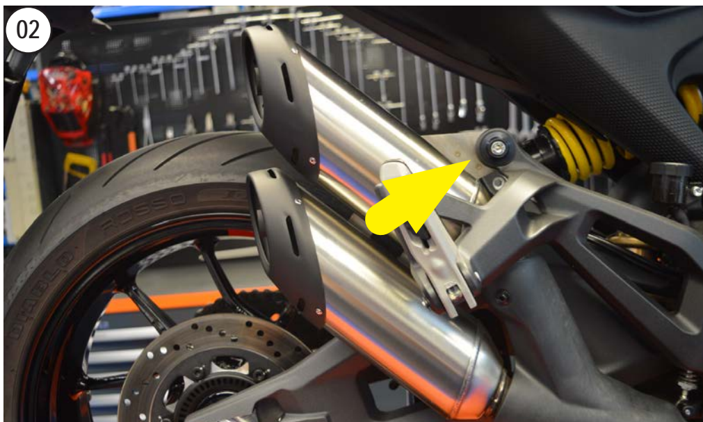
UNSCREW - REMOVE THE FASTENERS (Ducati Monster 937)
