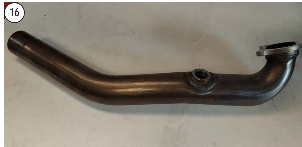
REMOVE THE FRONT PRIMARY PIPE
