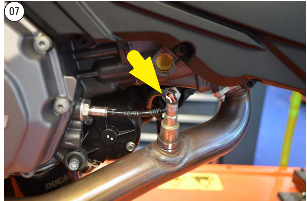
REMOVE THE LAMBDA SENSOR
