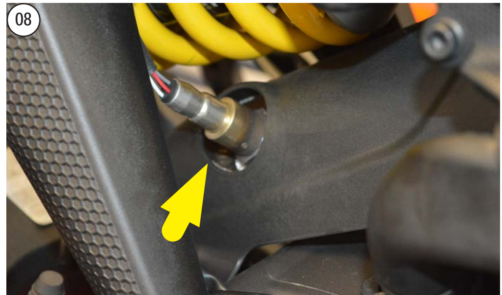
REMOVE THE LAMBDA SENSOR
