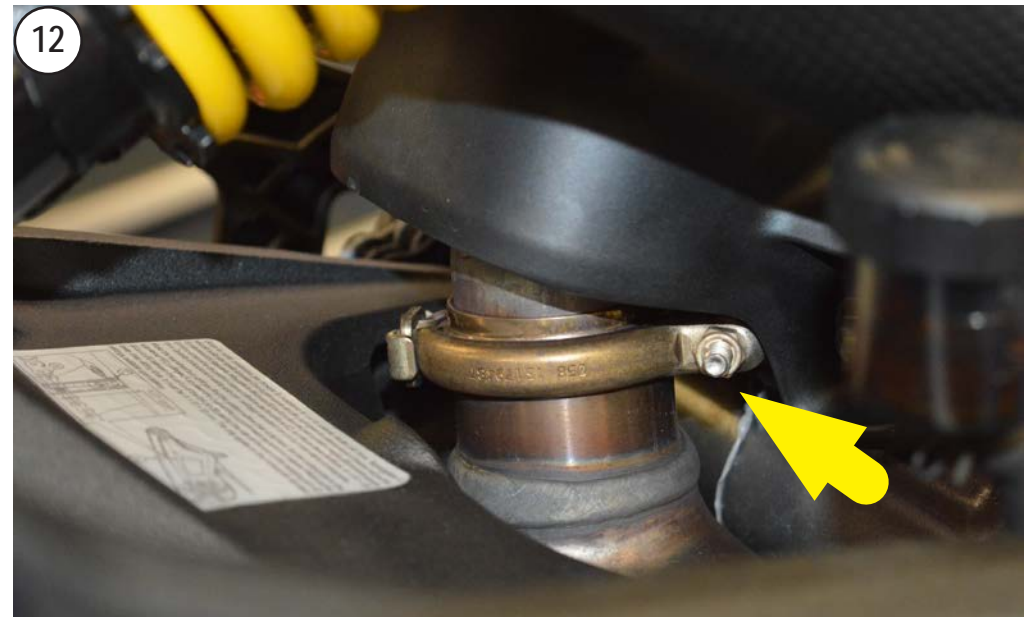
REMOVE THE CLAMP NEAR THE REAR DAMPER
