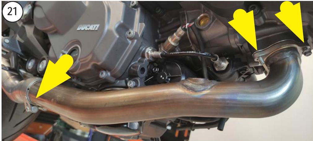
INSTALL THE FRONT PRIMARY PIPE
