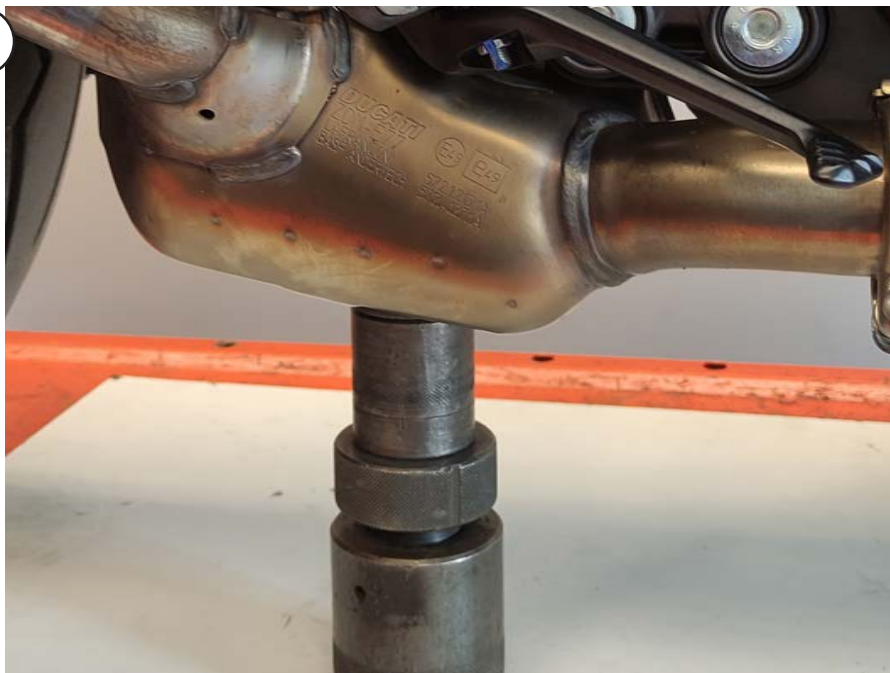
ATTENTION: PREVENT THE MIDPIPE TO FALLING DOWN
