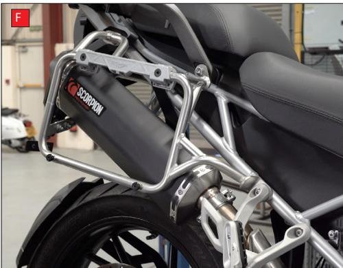
F) Slide the silencer onto the original exhaust pipe and line the bracket up with the original mounting point.
