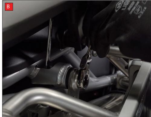
A) Loosen the clamp on the rear silencer.
