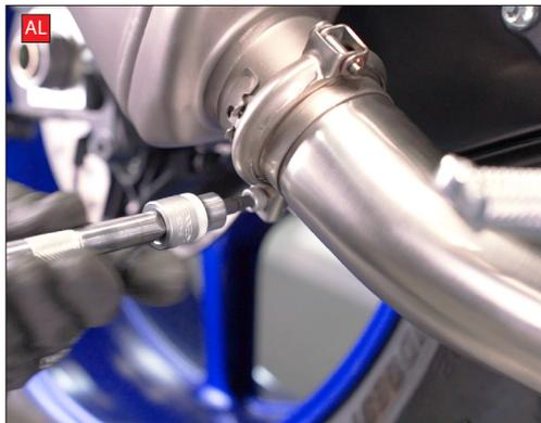
AM) Fully tighten the silencer mounting bolt.
