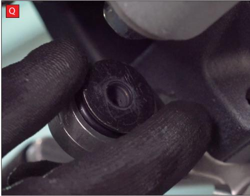
Q) Remove the sleeve from the left rear mount.
