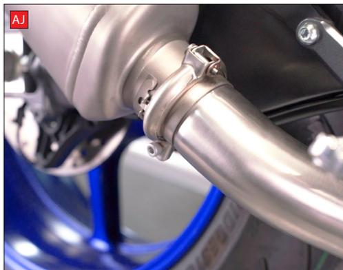
AJ) Re-fit the original clamp but leave loose at this point, you will fully tighten in a later step.
