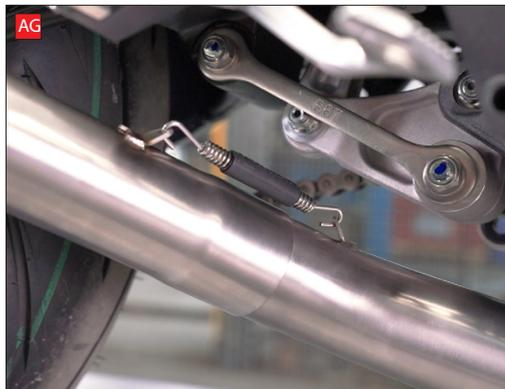
AG) Install the spring between the 2 pipes.
