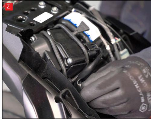
Y) Disconnect the cables from the motor.
