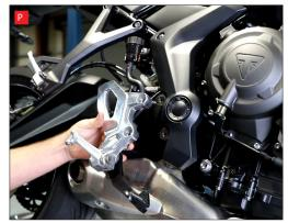
I) On the left side of the bike remove the 2 side panel mounting screws
