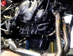
Q) Support the silencer from underneath, then remove the silencer mounting bolt.
