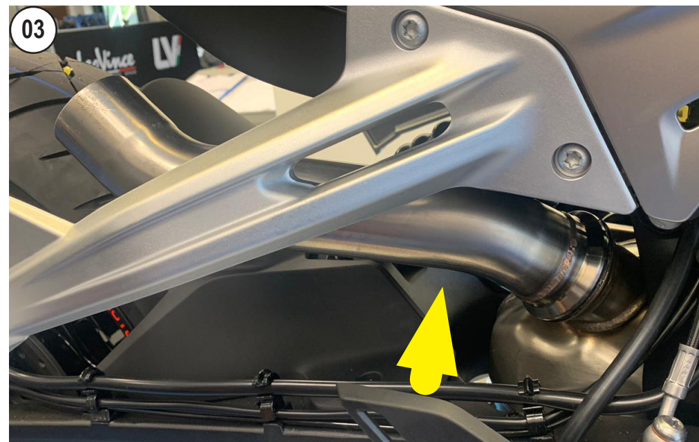
INSTALL THE LeoVince PIPE
