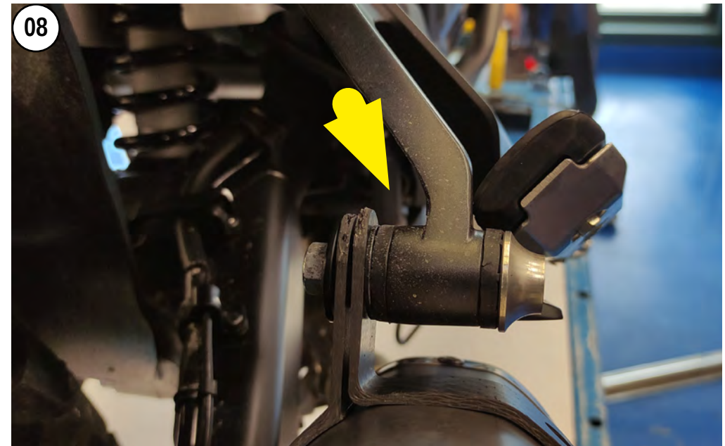
STACKING OF THE FASTENERS
