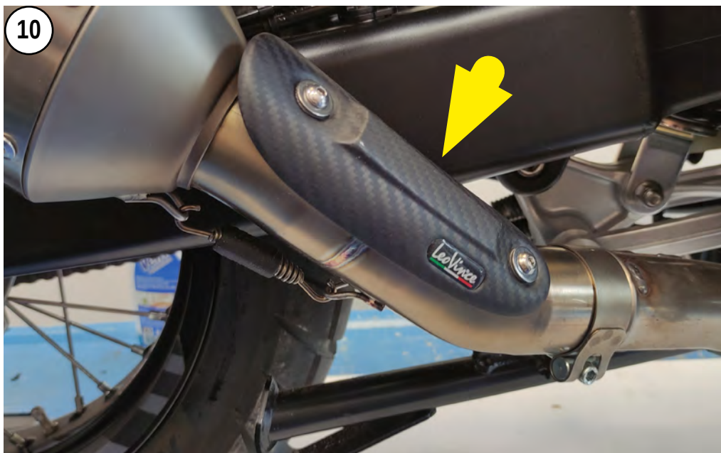
INSTALL THE CARBON HEAT SHIELD WITH ITS FASTENERS
