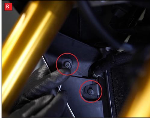
A) Remove the 2 mounting bolts for the fairings.
