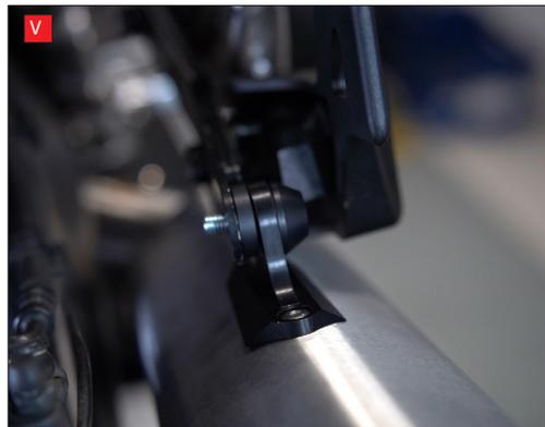
U) If your bike has pannier mounts you will need to use the supplied spacer between the mounting bracket and the silencer. If your bike hasn't got pannier mounts you will not need to use the spacer.
