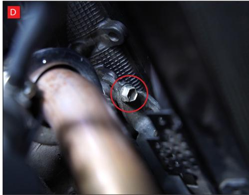
D) Remove the radiator support bracket bolt on the front of the engine.
