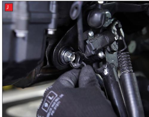
I) Remove the header nuts.
