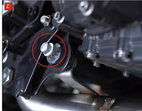
Y) Fully tighten header nuts.
