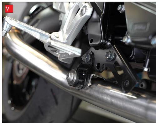
X) Slide the Scorpion silencer onto the connecting pipe and align with the mounting bracket.
