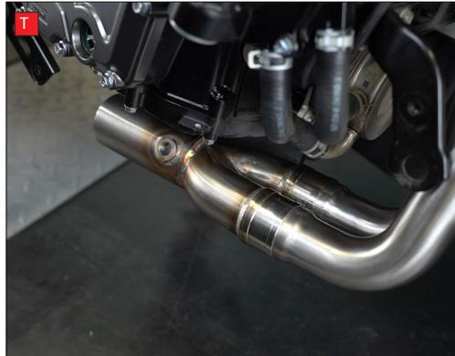
U) Slide the connecting pipe onto the collector and align the bracket with the mounting point on the frame.
