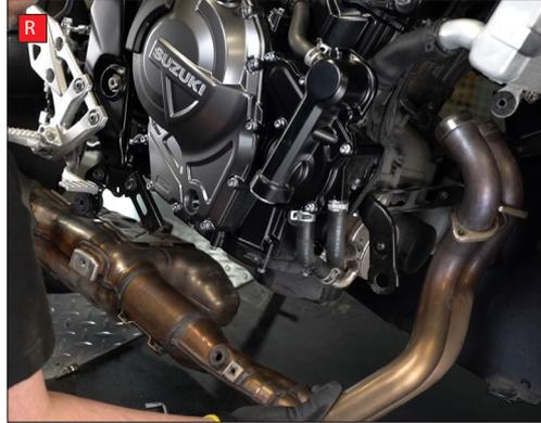
Q) On the right side of the bike support the weight of the exhaust and remove the mounting bolt.
