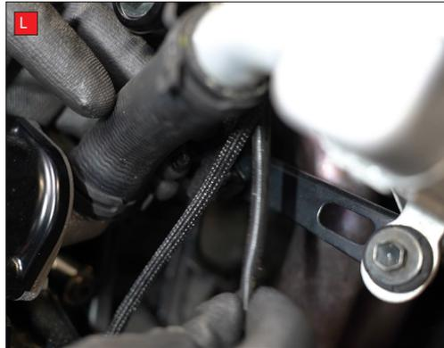
N) Completely remove the radiator support bracket.
