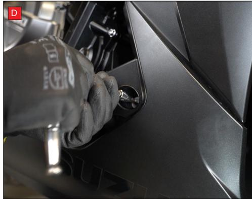
H) Carefully pull the fairing away from the bike to get to the indicator wiring.
