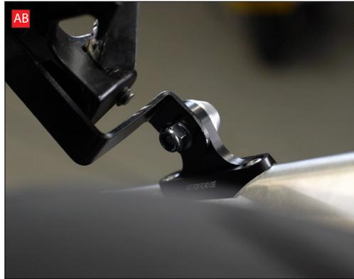
AB) Fully tighten the silencer mounting hardware.
