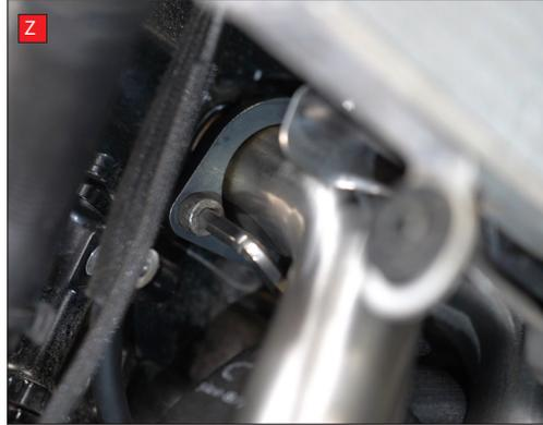
Y) Secure in place with the supplied hardware. Do not fully tighten yet, you will do this in a later step.
