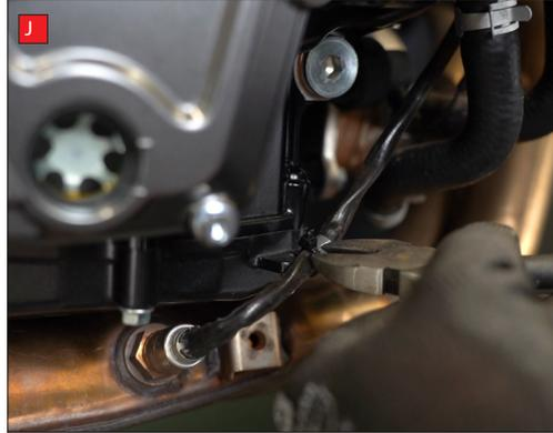
I) Disconnect the indicator wiring at the plug, you can then remove the fairing from the bike and put in a safe place.
