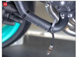
AD) Connect the extension harness to the plug and run behind the frame and engine mount, down towards the gear selector area with the breather hoses.
