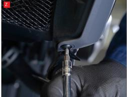
Y & Z) On the left side of the bike, remove the 2 bolts that hold the front/side plastic panel on.
