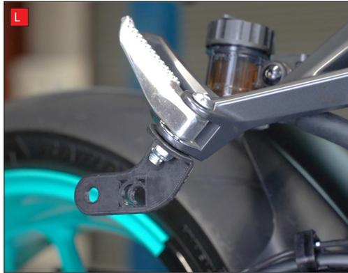
L) Attach the Scorpion mounting bracket with the supplied nut. Do not fully tighten, you will do that in a later step.
