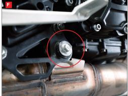
A) Remove both Lambda sensors from the original exhaust.
