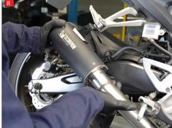
Q) Slide the Scorpion connecting pipe with the clamp onto the header pipe.
