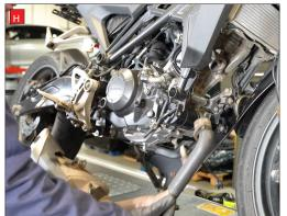
A) On the right hand side of the bike, remove the bolt from the back of the lower fairing.
