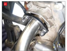
I) Remove both Lambda sensors from the original exhaust.
