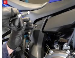
A) Remove the heat shield from the catalyst.
