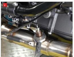
Q) Adjust the system if necessary, then fully tighten the header nuts.
