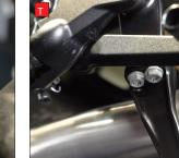
W) Refit the heat shield to the cat.
