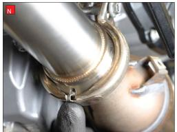
O) Slide the silencer onto the Scorpion delete pipe and line the mounting bracket up with the mount on the frame.
